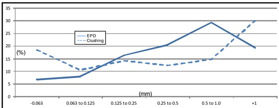
**Figure 4 – Average grain size distribution (proportion) of granitoid samples disaggregated by EPD and mechanical crushing.** The test included two sets of five granitoid samples and six quartz-vein blanks inserted before and after each sample.
