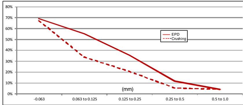
**Figure 5 – Average proportion of intact versus broken zircon grains extracted from the granitoid test samples.** The test included two sets of five granitoid samples and six quartz-vein blanks inserted before and after each sample.
