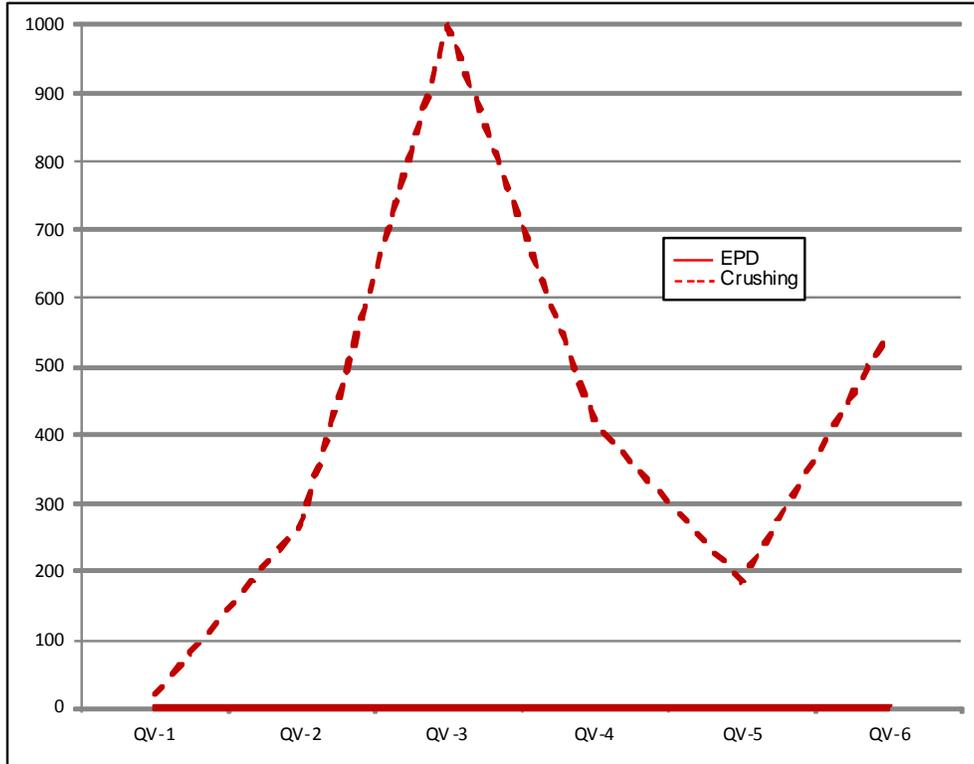
**Figure 3 – Number of zircon grains in blank samples after disaggregation.** The test included two sets of five granitoid samples and six quartz-vein blanks inserted before and after each sample.
