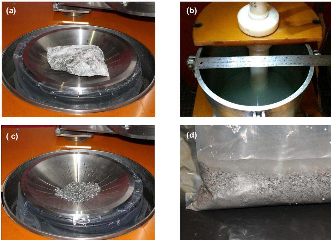
Figure 2 – EPD of rock sample. (a) Rock on stainless steel sieve; (b) electrode placed into water-filled, large capacity disaggregation chamber; (c) +1 mm, post EPD fragments; and (d) -1 mm, post EPD mineral grains in sample bag with process water.
