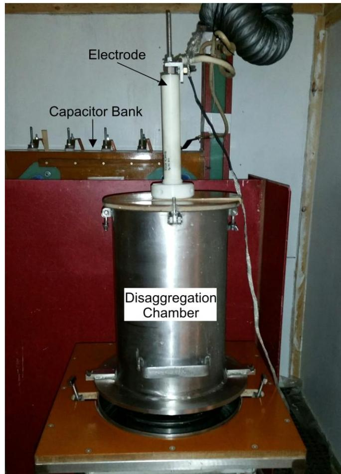
Figure 1 – ODM’s Spark-2 Electric-Pulse Disaggregator (“EPD”).
